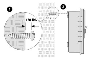
3 Remove the wiring bay cover on the lower part of the controller unit, and drive a second screw through the open hole inside the controller and into the wall, as shown.
