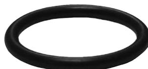
In order to ensure the highest degree of safety at all times, it is important that the gasket compression is not linked to ring nut torque, otherwise this would cause the risk of leaks due to incorrect torque of the fitting or release of the ring nut when subjected to pressure cycles. Unidelta fittings are equipped with an O-Ring seal placed firmly in a cylindrical seat and do not require any compression rings.
