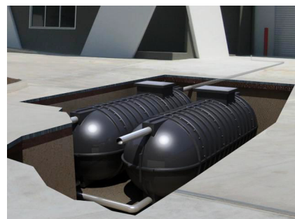
Low level interconnecting pipework
