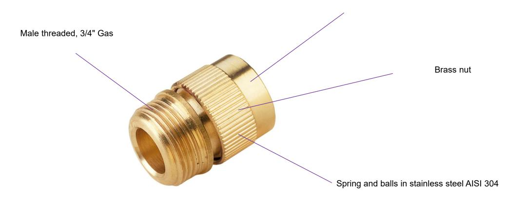
Temperature min/max.-20°C +80°C Working pressure max. 10 bar
