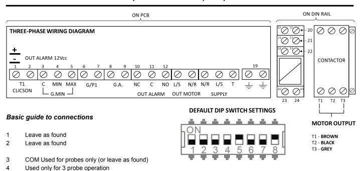
6 Connection from additional Pressure Switch or Floatswitch (or leave as found)
