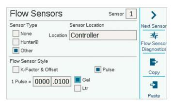
Pulse type: Enter the amount equal to a single pulse.
