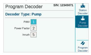
Enter the P/MV number for the decoder. This must match the P/MV assignment in the Devices menu.
