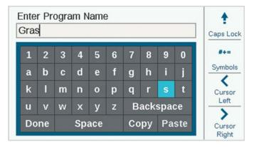
Select the Name field for any of these components, and a keyboard will appear to enter an alphanumeric name.
