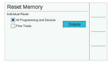
**All Programming and Devices:** This erases all programs and device setups, but keeps the Flow Totals intact.
