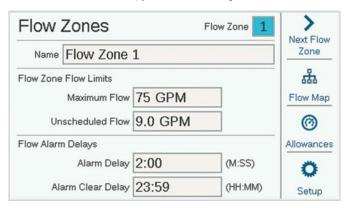
**Maximum Flow:** This sets the highest possible flow rate allowed in the Flow Zone for any reason. This should be considerably larger than the maximum flow allowed in normal irrigation (so that it does not alarm before station-level diagnostics can be performed). When the flow sensor detects a flow higher than this, the irrigation will be shut down.
