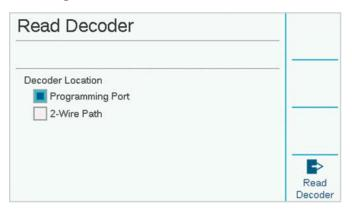
Then press the soft key labeled Read Decoder. This will return the configuration of the decoder in the port, with a screen for entering the station numbers. If the screen says "Decoder Not Found!" the decoder wires may be disconnected, or the wrong wires may have been inserted.
