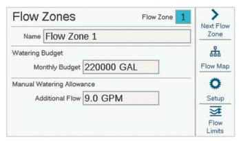
Watering Budget: Enter the total amount of flow that can be allowed in this Flow Zone in the calendar month. If the total flow exceeds the monthly budget, an alarm message will appear on the screen. The controller will not automatically stop watering when this alarm occurs.
