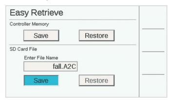
**Controller Memory:** Only one setup may be saved in Controller Memory, and it will remain unless you make changes and create a new Easy Retrieve backup in the future. You can choose Restore at any time, and it will change the whole controller to the last Easy Retrieve backup.
