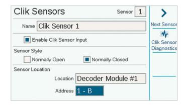
To set up a sensor, click the box for Enable Clik Sensor Input.
