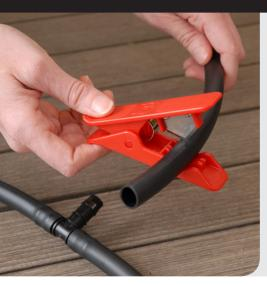
The Antelco Micro Irrigation Tube Cutter is ideal for cutting low pressure irrigation tubes for micro irrigation installations.
