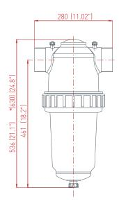
Dim. in mm (inch) \*Approx. length required for maintenance
